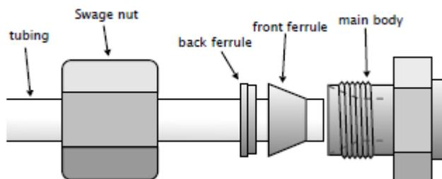
NOTE: Nylon ferrules only need to be tightened a little past finger tight (about 1/4 of a turn). Use caution, over tightening can damage the ferrule set.
