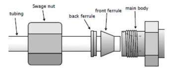
For nylon ferrules, fully insert the tube into the fitting and rotate the nut finger-tight. Tighten the nut an additional approximately 1/8 turn past finger tight.
